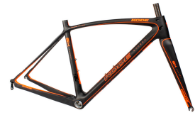
448-QUADRO KODE SK CARBON ROAD PTO/LARANJA FLUO P. FIT 41X86.5MM/TAPERED/SUP. SELIM 27.2
